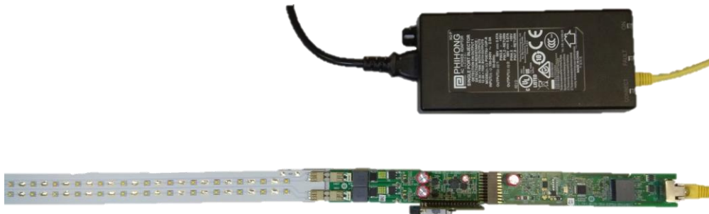
Figure 5. Lighting Platform Hardware Setup with PoE power supply
